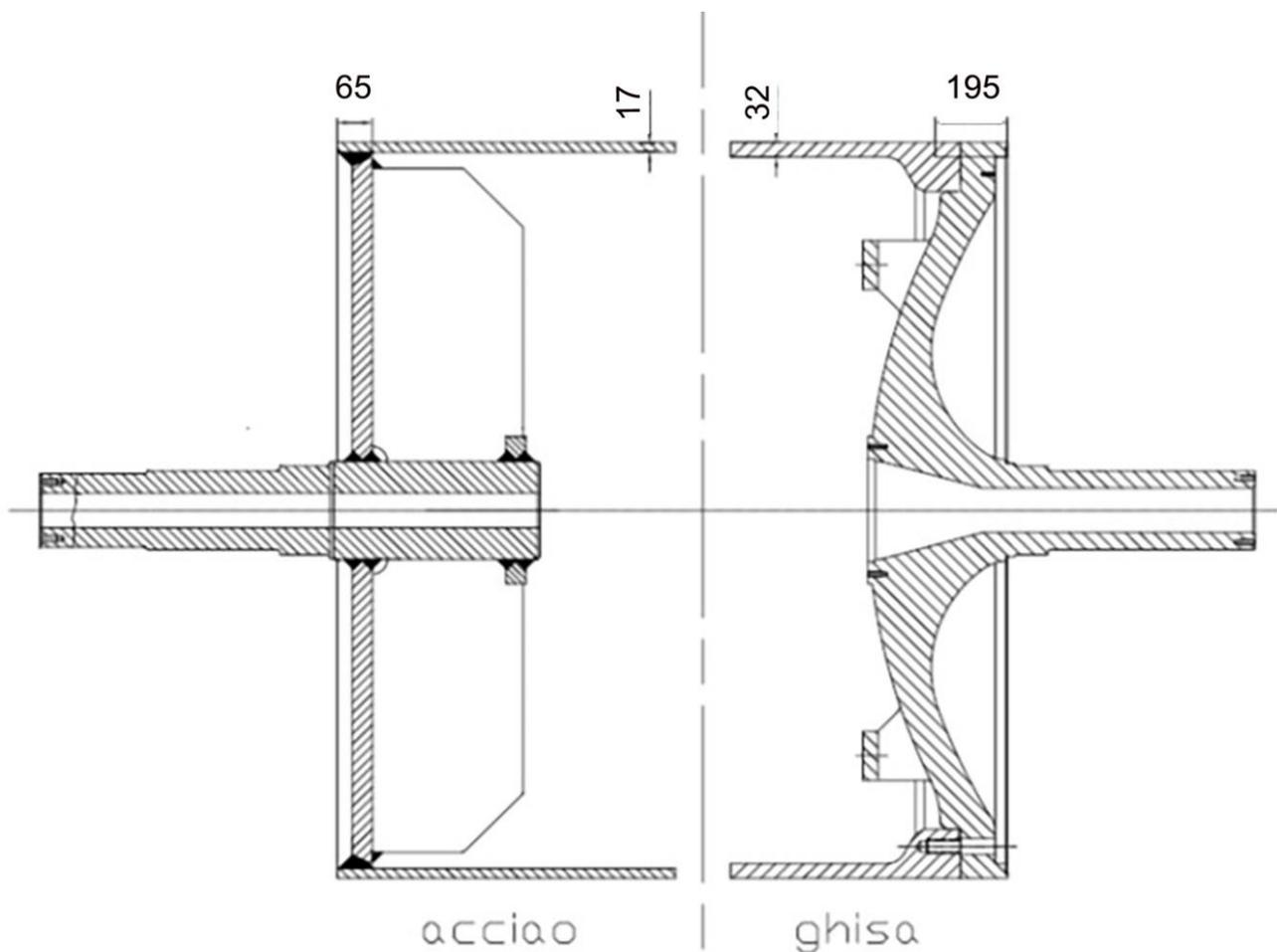
*FIGURE 2: Construction drawing of steel (left) and cast iron (right) drying cylinders.*
