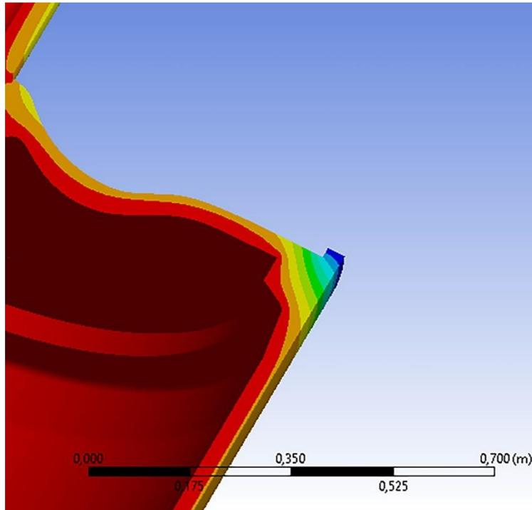
*FIGURE 6: Trend of temperatures in the thickness of the G25 cast iron dryer cylinder.*
