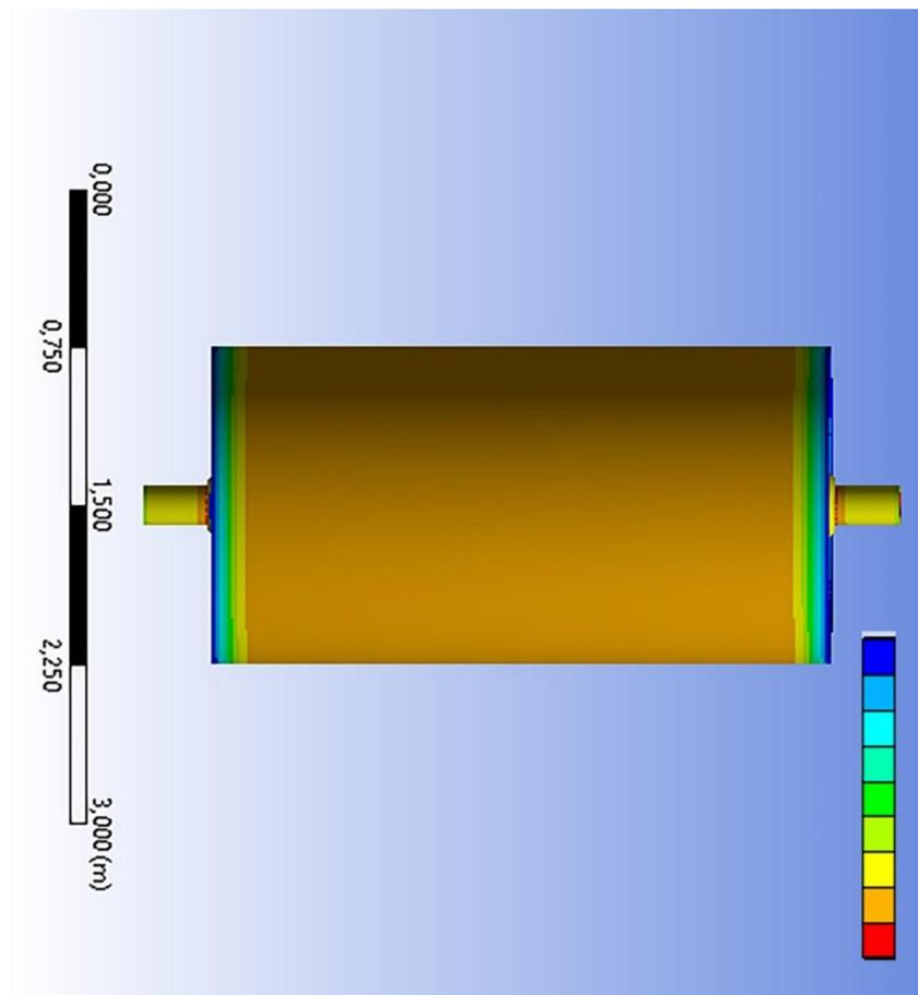
*FIGURE 5: Trend of temperatures on the shell of the G25 cast iron dryer cylinder.*
