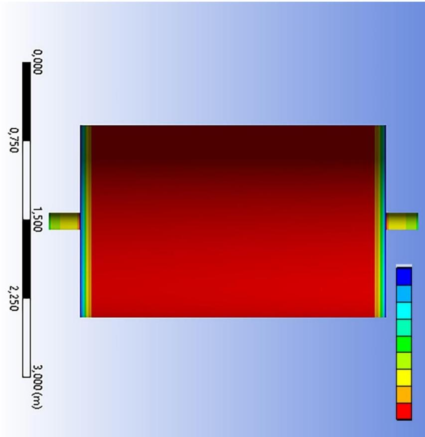
FIGURE 3: Trend of temperatures on the shell of the P275NH steel dryer cylinder.
