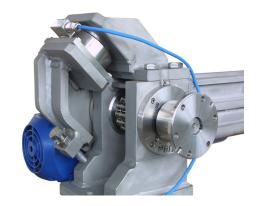
The felt / wire line adjustment in the TC stretch-compensators is carried out by a screw-jack which limits the adjustment field of the roll and at the same time measures its misalignment. This adjustment can be manual or motorized and the measure of misalignment can be visual or remote-controlled for the sections of machine which are less accessible.
