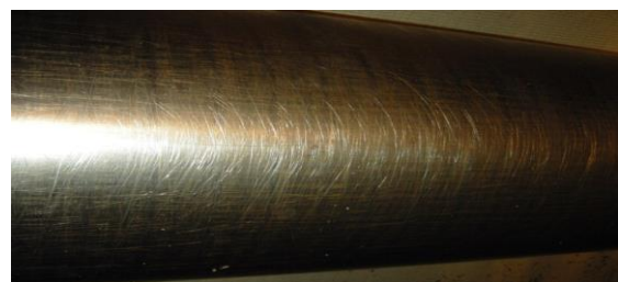
Fig. 8 Fabric rolls 6 months after cleaning
